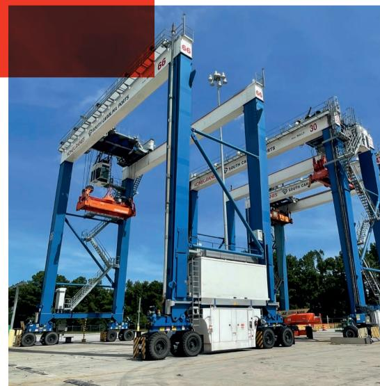
Retrofits on RTGs at the Wando Welch Terminal have reduced emissions, energy consumption and maintenance requirements.
